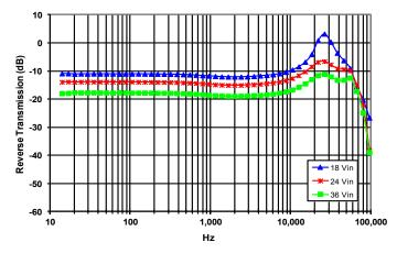
Figure 21: Magnitude of incremental reverse transmission ( $RT = i_{ii}/i_{out}$ ) for minimum, nominal, and maximum input voltage at full rated power.
