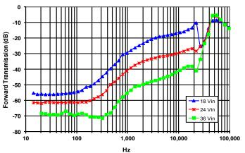
Figure 20: Magnitude of incremental forward transmission ( $FT = v_{oul}/v_{u}$ ) for minimum, nominal, and maximum input voltage at full rated power.
