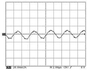
Figure 15: Input reflected ripple current,  $i_s$ , through a 3.3  $\mu$ H source inductor at nominal input voltage and rated load current (20 mA/div). See Figure 13.
