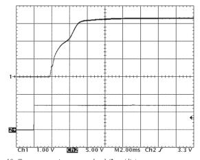
Figure 10: Turn-on transient at zero load (2 ms/div). Ch 1: Vout (1V/div) Ch 2: ON/OFF input (5V/div)
