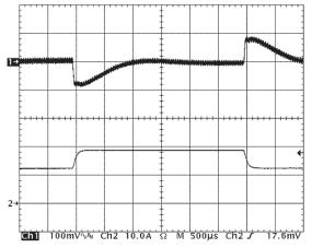
Figure 11:Output voltage response to step-change in load current (50%-75%-50% of lout(max);  $dI/dt = 0.1A/\mu s$ ). Load cap:  $10\mu F$ , 100 m $\Omega$  ESR tantalum capacitor and  $1\mu F$  ceramic capacitor. Ch 1: Vout (100mV/div), Ch 2: lout (10A/ div).
