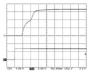
Figure 9: Turn-on transient at full load (resistive load) (2 ms/div). Input voltage pre-applied. Ch 1: Vout (1V/div). Ch 2: ON/OFF input (5V/div)
