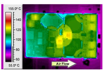
Figure 6: Thermal plot of converter at 20 amp load current with  $55^{\circ}$ C air flowing at the rate of 200 LFM. Air is flowing across the converter from input to output (nominal input voltage).
