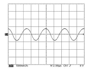
Figure 14: Input Terminal Ripple Current,  $i_c$ , at full rated output current and nominal input voltage with 3.3 $\mu$ H source impedance and 100 $\mu$ F electrolytic capacitor (500 mA/div). See Figure 13.
