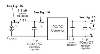
Figure 13: Test set-up diagram showing measurement points for Input Terminal Ripple Current (Figure 14), Input Reflected Ripple Current (Figure 15) and Output Voltage Ripple (Figure 16).
