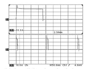
Figure 18: Load current (10A/div) as a function of time when the converter attempts to turn on into a 10 m $\Omega$  short circuit. Top trace (2.5ms/div) is an expansion of the on-time portion of the bottom trace.
