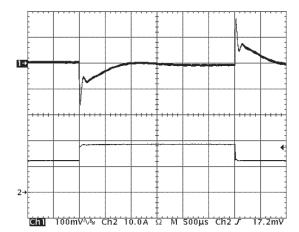
Figure 12: Output voltage response to step-change in load current (50%-75%-50% of Iout(max):  $dI/dt = 5A/\mu s$ ). Load cap:  $470\mu F$ ,  $30 \ m\Omega \ ESR$  tantalum capacitor and  $1\mu F$  ceramic cap. Ch 1: Vout (100mV/div), Ch 2: Iout (10A/div).
