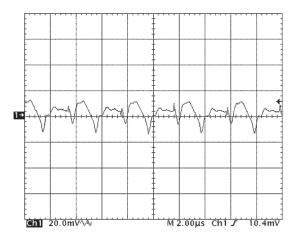
Figure 16: Output voltage ripple at nominal input voltage and rated load current (20 mV/div). Load capacitance:  $1\mu$ F ceramic capacitor and  $10\mu$ F tantalum capacitor. Bandwidth: 20 MHz. See Figure 13.
