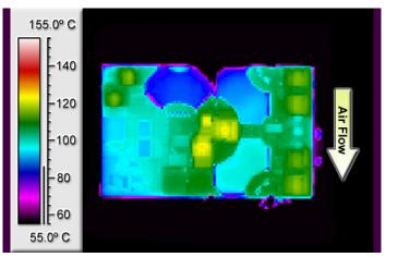
Figure 8: Thermal plot of converter at 19 amp load current with  $55^{\circ}$ C air flowing at the rate of 200 LFM. Air is flowing across the converter from pin 1 to pin 3 (nominal input voltage).
